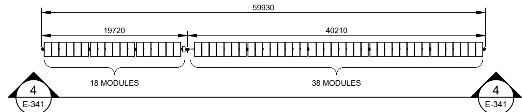
2 TYPICAL ARRAY PLAN - 56 MODULE TRACKER SCALE: 1:500
